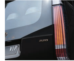
Parametric Pixel Light (LED Rear Combination Lamps)
